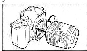
2 Align the red dots on the camera and lens mount, attach the lens to the camera body, and turn it fully to the right until it clicks into place.
